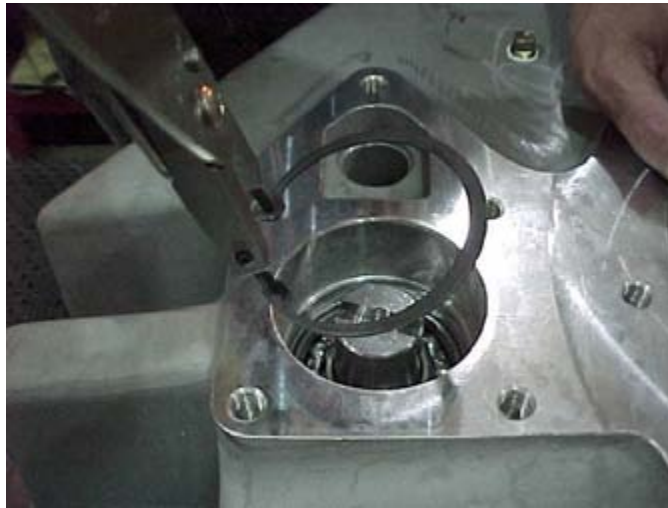
Figure 62. Installing Internal Retaining Ring
