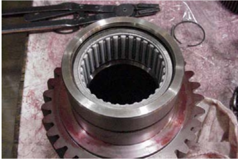
Figure 78. Needle Roller Bearing Installed
