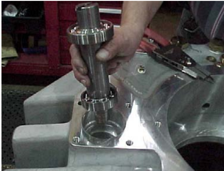
Figure 30. Removing Shaft Assembly
