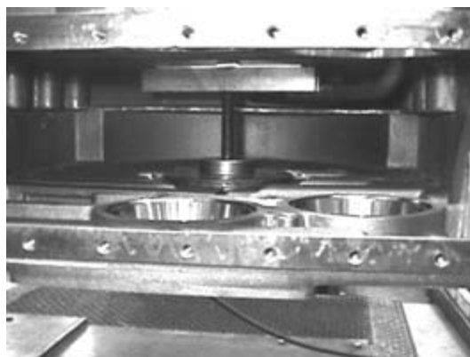
Figure 59. Installing Output Shaft Front Bearing
