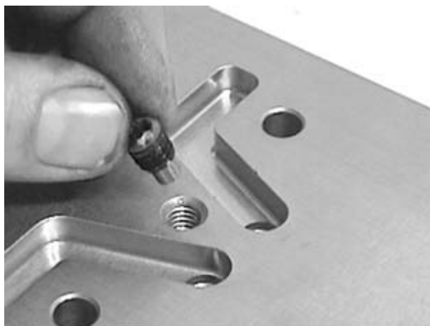
Figure 116. Installing Dogpoint Setscrew
