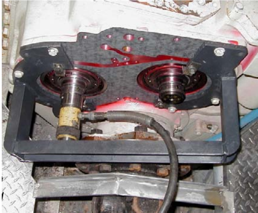
Figure 90. Fixture Used to Establish Secondary Shaft Bearing Clearance
