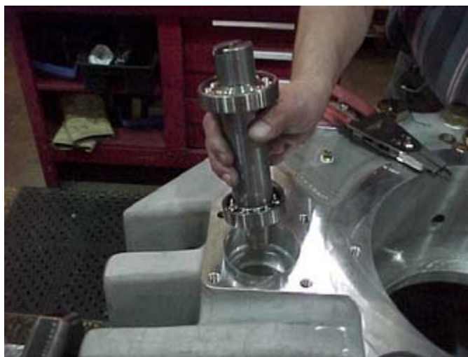
Figure 61. Installing Trailing Pump Shaft
