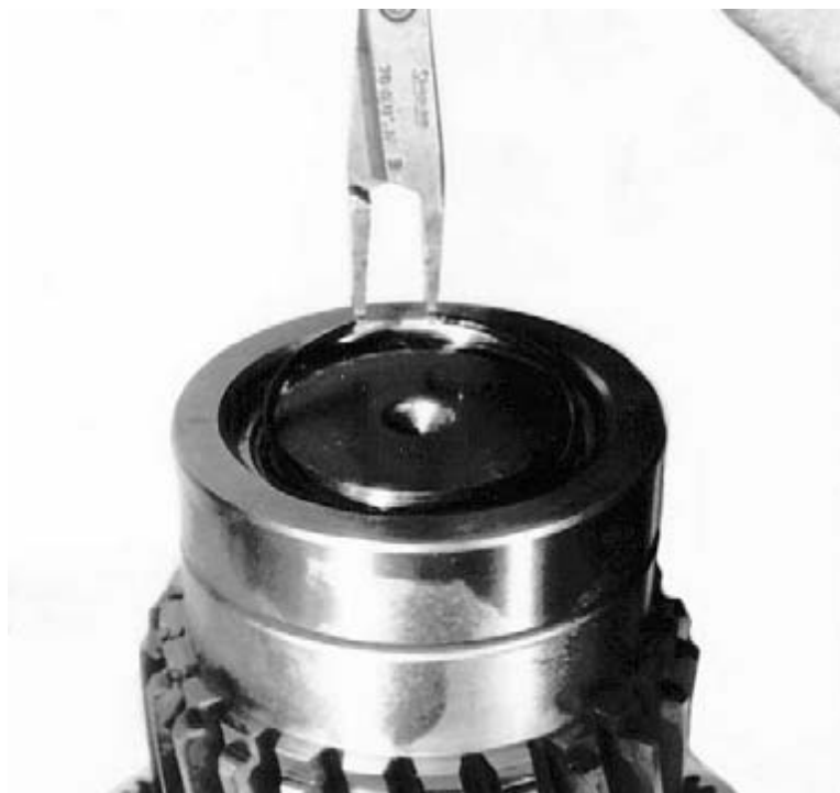
Figure 32. Removing Round Retaining Ring from Input End of Shaft
