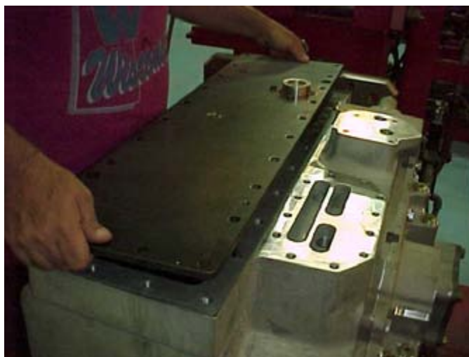
Figure 111. Installing Top Cover
