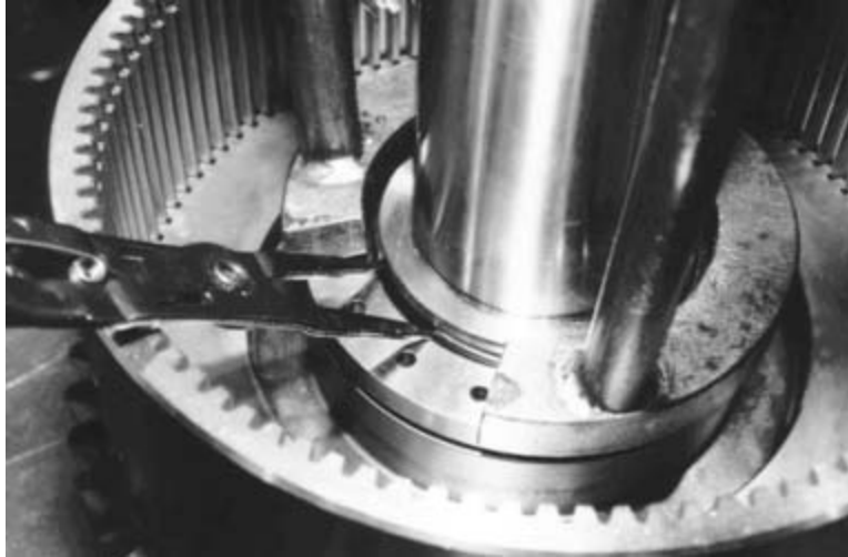
Figure 92. Installing Spring Retainer Retaining Ring
