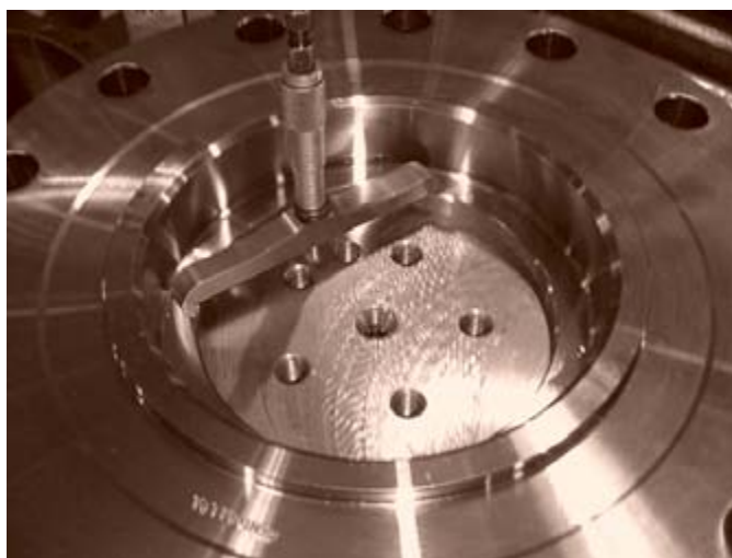
Figure 108. Measuring Output Step Height
