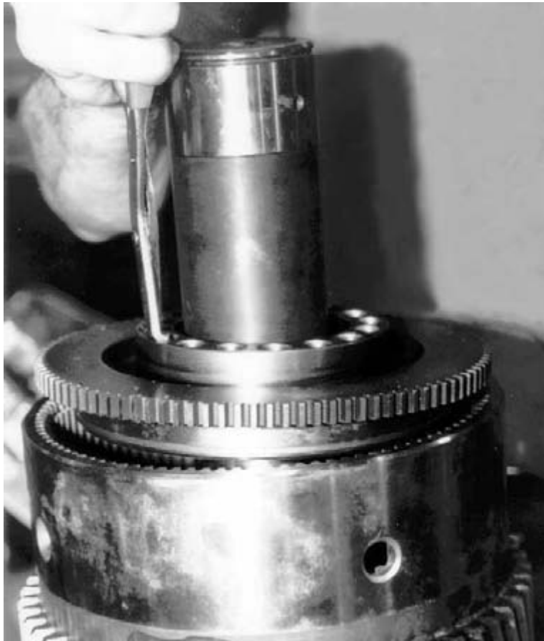
Figure 76. Installing Clutch Piston
