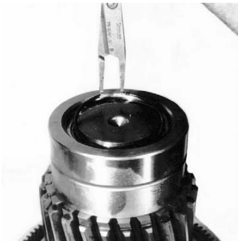
Figure 36. Removing Round Retaining Ring from Input End of Shaft
