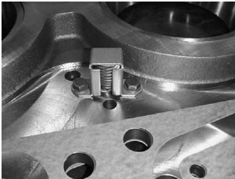
Figure 88. Lubrication Oil Pressure Relief Valve Installed
