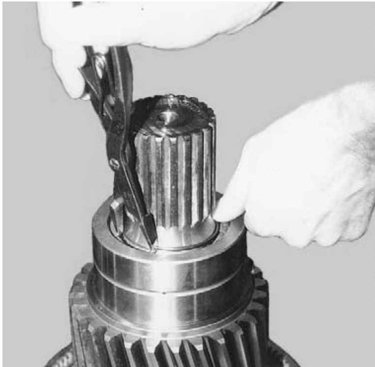
Figure 87. Installing External Retaining Ring Onto Clutch Shaft
