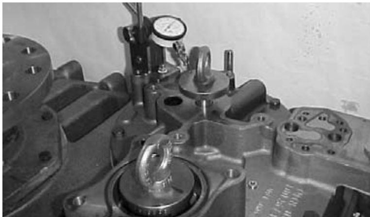
Figure 102. Confirming Secondary Shaft Bearing Adjustment
