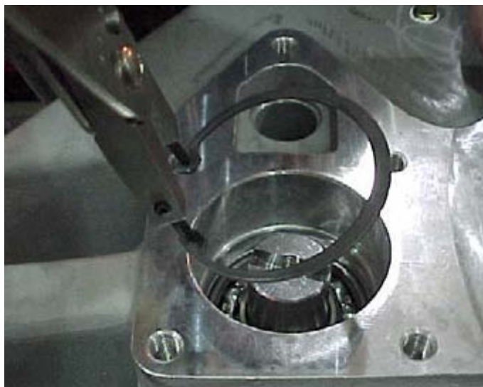
Figure 29. Removing Internal Retaining Ring
