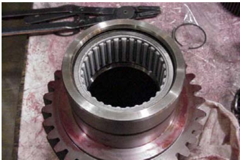
Figure 95. Needle Roller Bearing Installed
