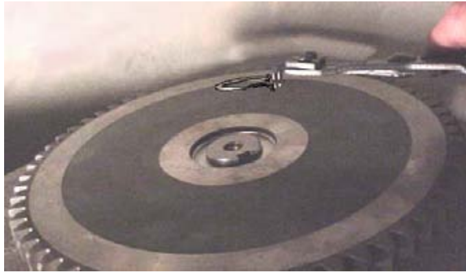
Figure 28. Removing External Retaining Ring
