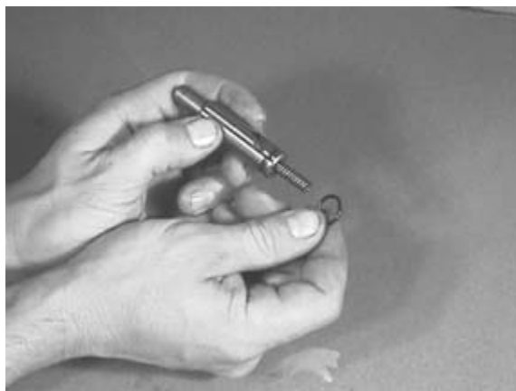
Figure 54. Removing O-ring from Stem
