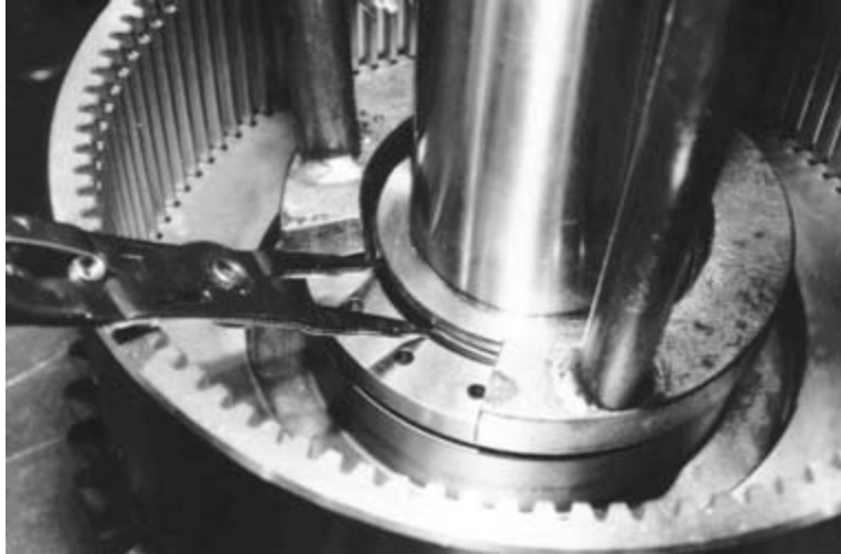
Figure 38. Removing Spring Retainer Retaining Ring
