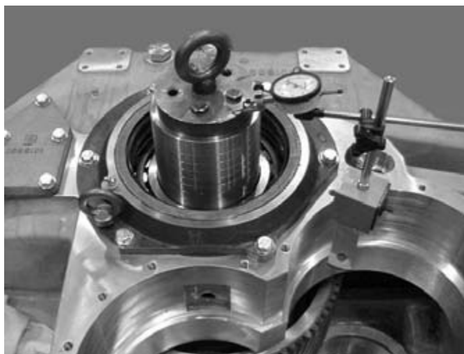
Figure 69. Measuring Output Shaft Endplay
