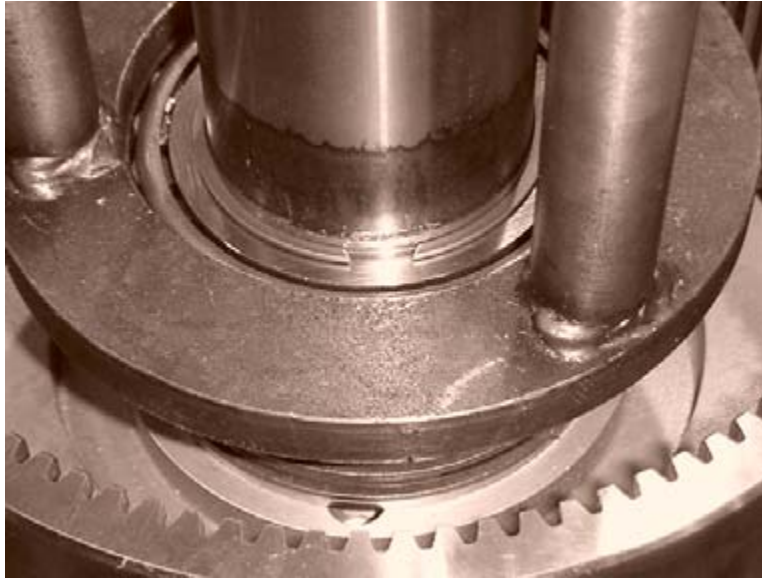
Figure 85. External Retaining Ring Installed
