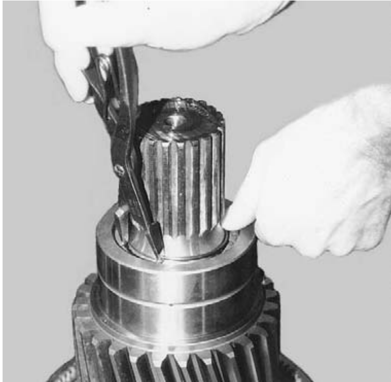
Figure 80. Installing External Retaining Ring Onto Clutch Shaft
