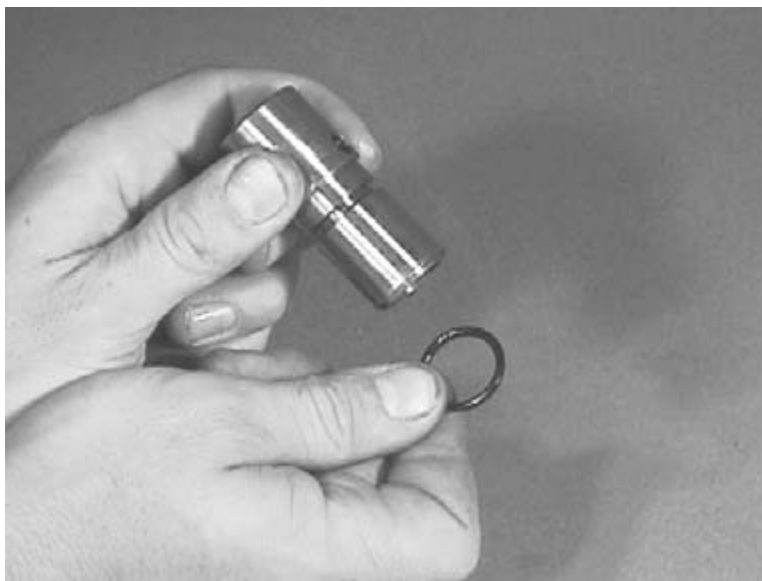
Figure 121. Installing O-ring onto Adapter
