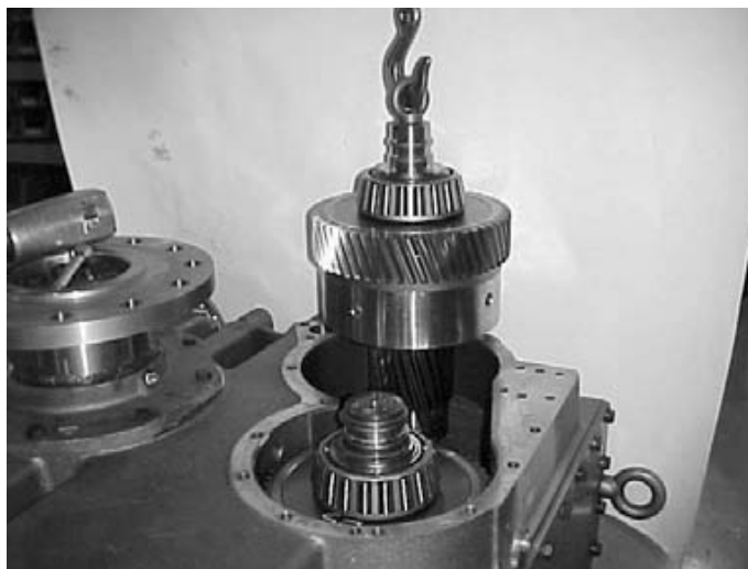
Figure 98. Installing Clutch Shaft Assembly
