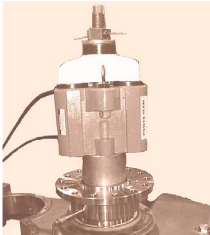
Figure 109. Advancing Output Flange Onto Output Shaft
