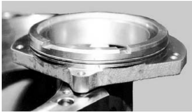
Figure 70. O-ring Installed onto Output Seal Carrier
