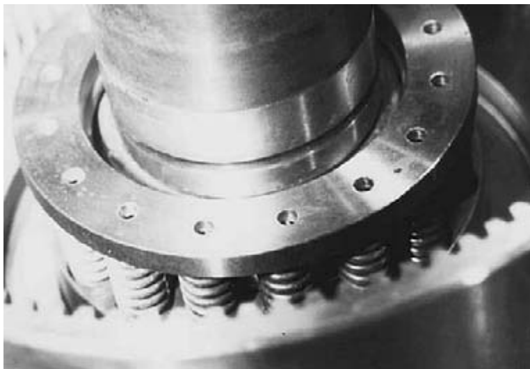
Figure 91. Return Springs and Spring Retainer Ready for Installation
