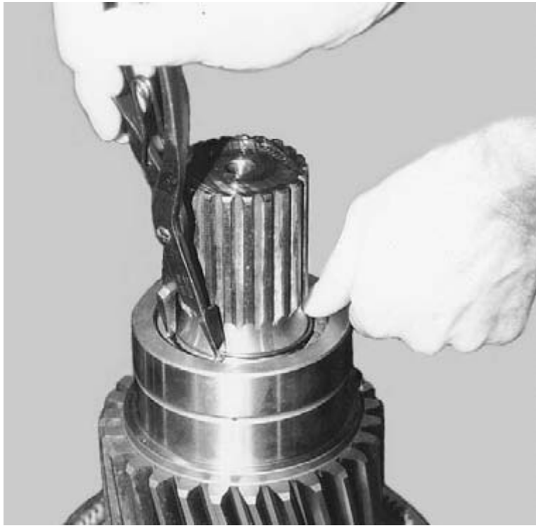
Figure 97. Installing External Retaining Ring Onto Clutch Shaft
