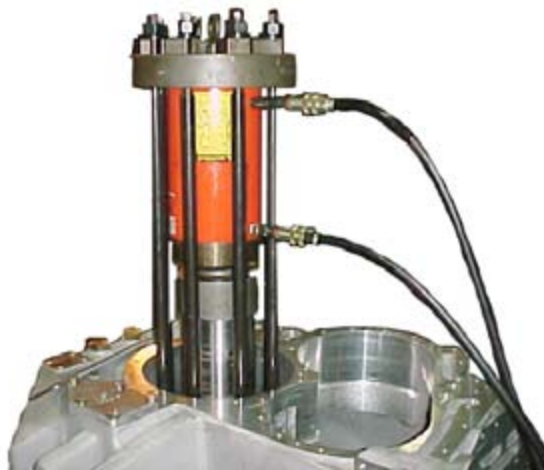
Figure 66. Advancing Output Gear
