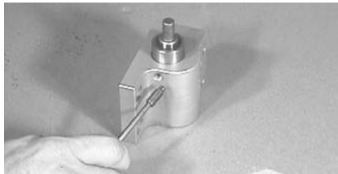
Figure 52. Removing Dogpoint Setscrew
