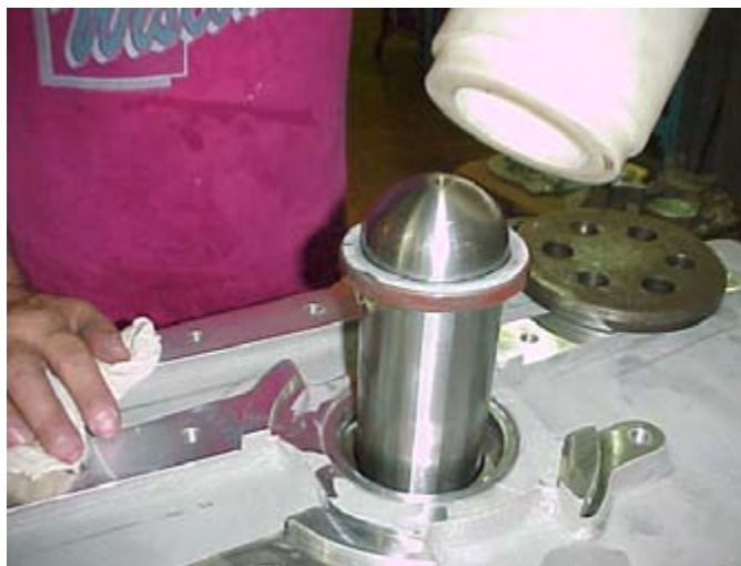
Figure 112. Installing Input Oil Seal
