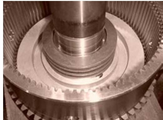
Figure 84. Correct Spring Stacking (left) and Installation (right)
