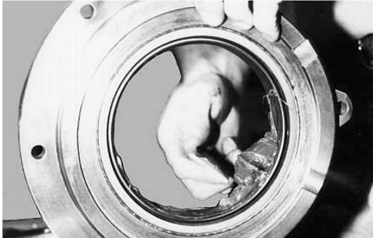
Figure 72. Packing Cavity Between Output Seals With Grease
