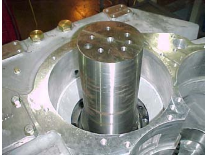
Figure 67. Output Bearing Cup Installed
