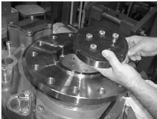
Figure 110. Installing Output Flange Retainer Washer and Shims
