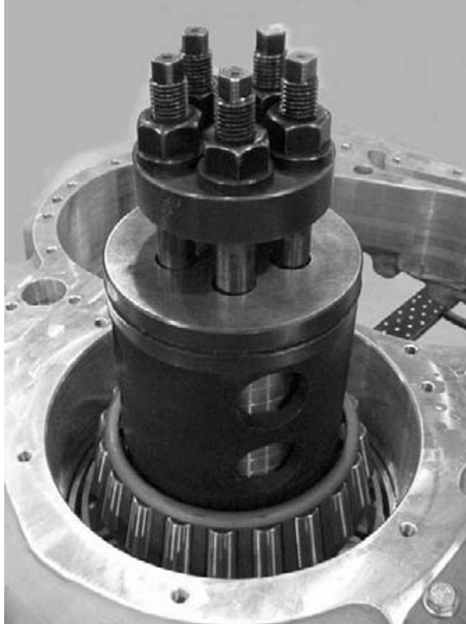
Figure 68. Output Bearing Tool T-21506
