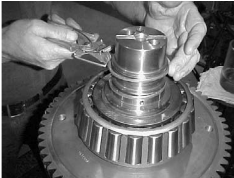
Figure 35. Removing Piston Rings From Shaft
