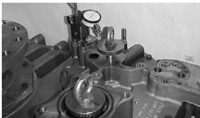
Figure 83. Confirming Secondary Shaft Bearing Adjustment
