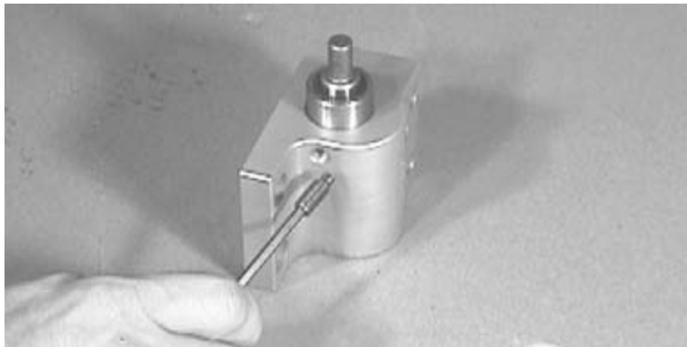
Figure 123. Installing Dogpoint Setscrew
