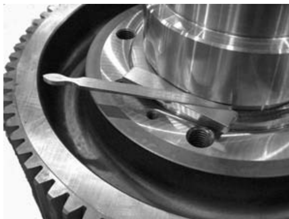
Figure 65. Measuring Output Gear Advance
