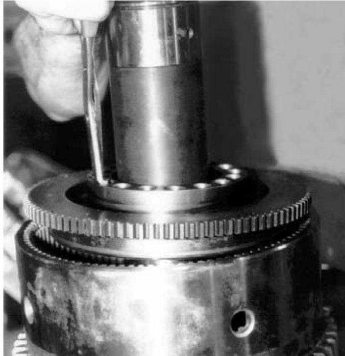
Figure 39. Removing Clutch Piston
