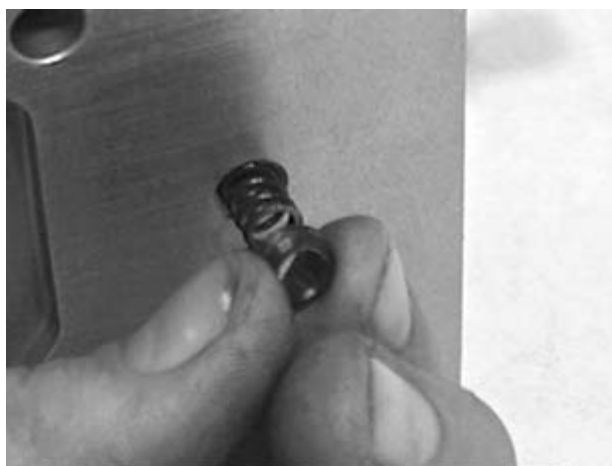
Figure 117. Installing Detent Ball Setscrew
