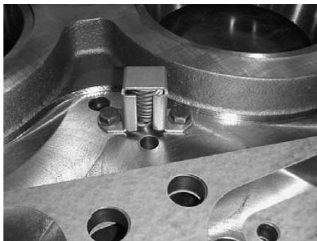
Figure 99. Lubrication Oil Pressure Relief Valve Installed
