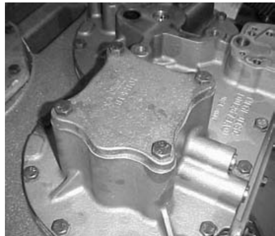
Figure 104. O-ring Installed (left) and Cover Installed (right)
