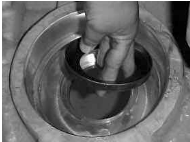
Figure 57. Seal Protector Installation
