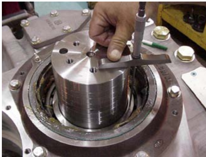
Figure 107. Measuring From Output Shaft Height
