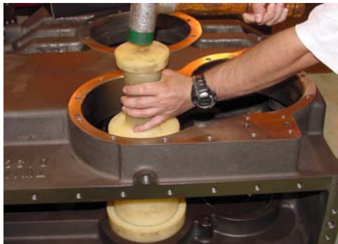
Figure 58. Front Pinion Bearing Cup Installation
