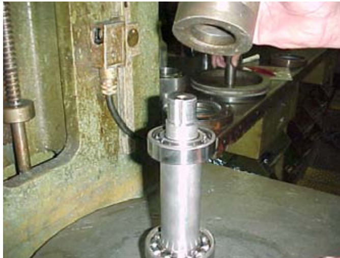
Figure 60. Installing Trailing Pump Shaft Bearings
