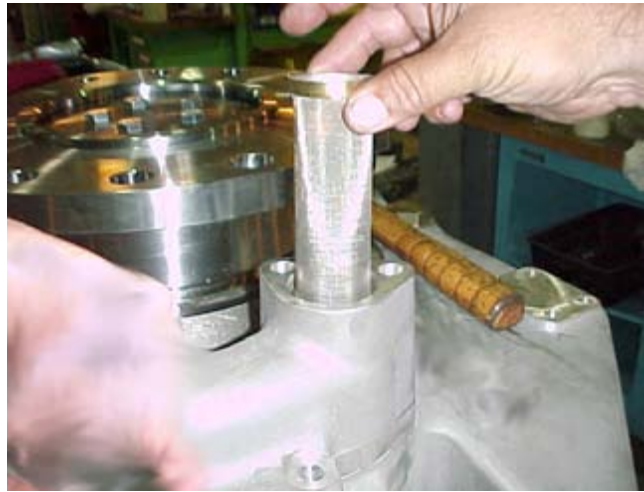
Figure 103. Installing Suction Strainer
