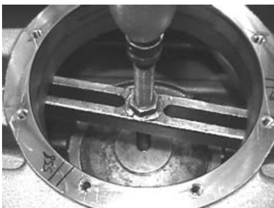
Figure 59. Installing Output Shaft Front Bearing
