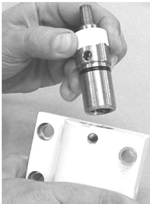
Figure 53. Removing Stem and Adapter from Valve Body (left) and Removing Stem from Adapter (right)
