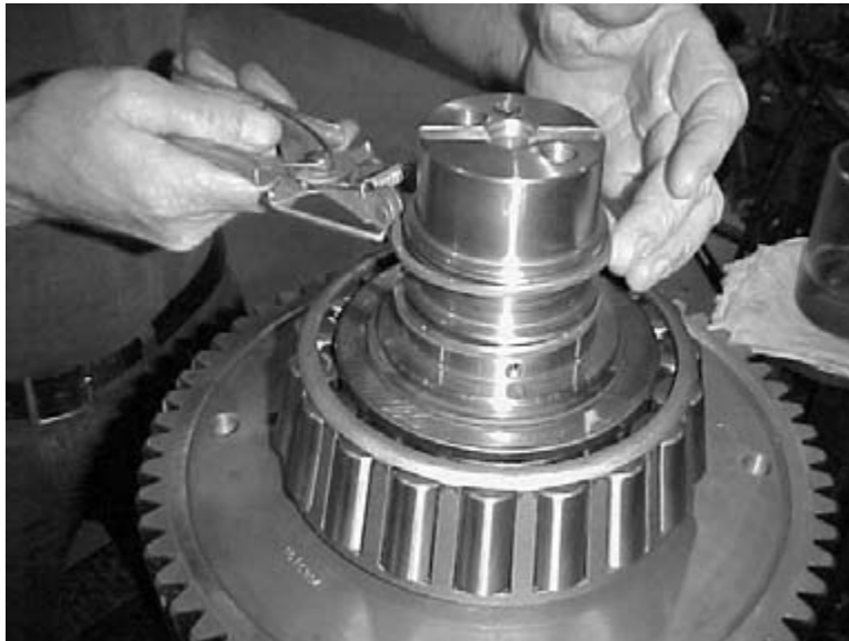
Figure 31. Removing Piston Rings From Shaft
