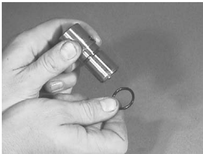
Figure 56. Removing O-ring from Adapter
