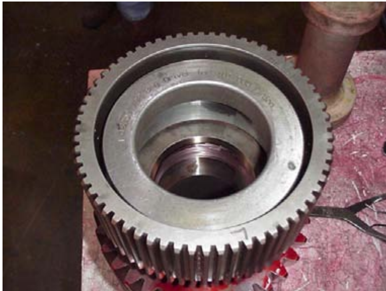
Figure 77. Installing Tapered Roller Bearing Cup Into Pinion
