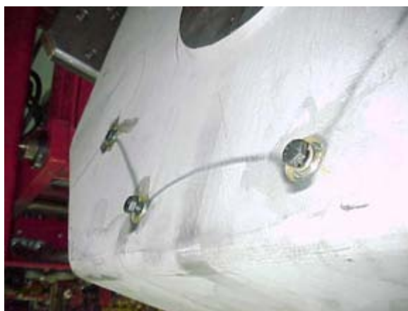
Figure 74. Installing Output Gear Pan Screws
