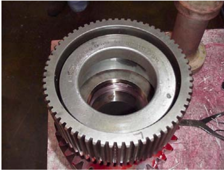
Figure 94. Installing Tapered Roller Bearing Cup Into Pinion
