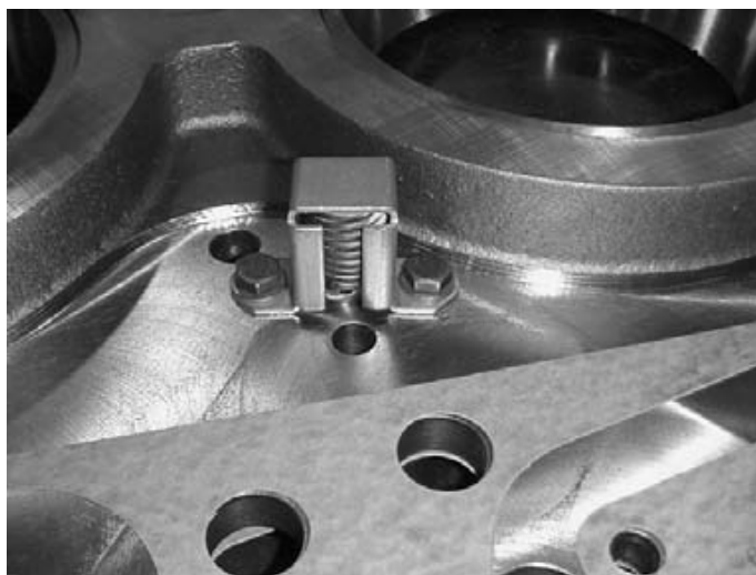
Figure 22. Lubrication Oil Pressure Relief Valve
