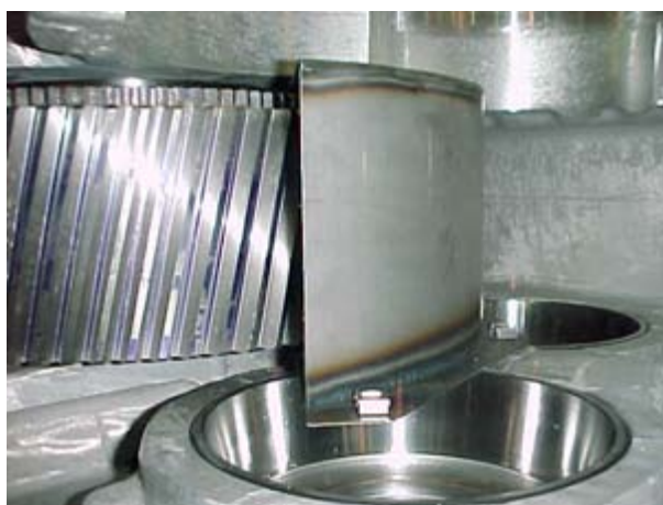
Figure 73. Installing Output Gear Pan
